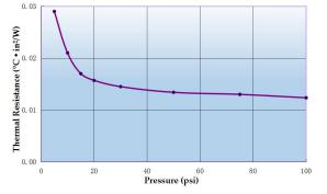
Flextein<sup>™</sup> PCM30 Thermal Resistance vs. Pressure
